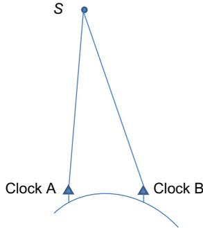
**Fig. 6** Use of common-view in GPS.
