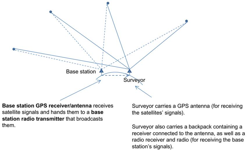
**Fig. 3** RTK surveying.
