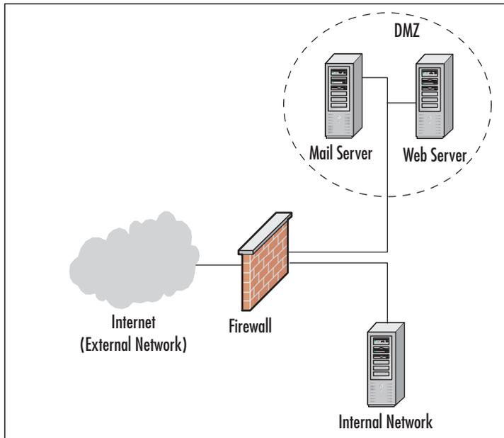
The role of the firewall in all of these scenarios is to manage the traffic between the network segments. The basic idea is that other systems on the Internet are allowed to access only the services of the DMZ systems that have been made
