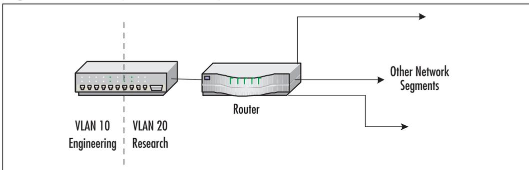
Each VLAN functions like a separate switch due to the combination of hardware and software features built into the switch itself. Thus, the switch must be
