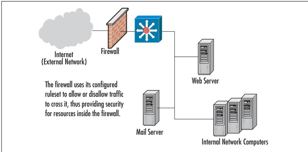
Many of these early firewalls had only basic abilities and usually functioned only as a packet filter. Packet filters rely on ACL's. ACL's allow the packet filter to be configured to block or allow traffic based on attributes such as IP address and source and destination port. Packet filters are considered stateless, while more advanced modern firewalls like Microsoft's ISA server is considered stateful. Regardless of what type of firewall you are working with, most provide the ability to:
