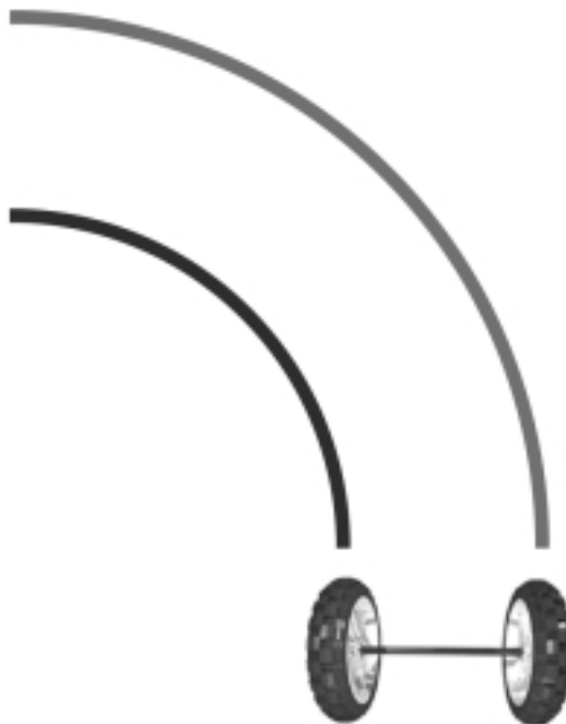
Figure 2.21 During Turns the Wheels Cover Different Distances
