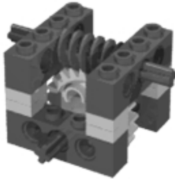
Figure 2.4 A Worm Gear Engaged with a 24t
