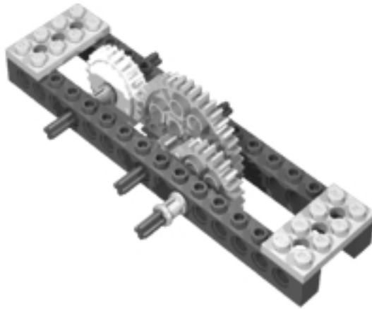
Figure 2.6 Placing the Clutch Gear in a Geartrain
