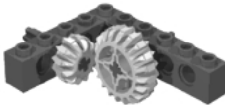
Figure 2.15 Double Bevel Gear on Perpendicular Axes
