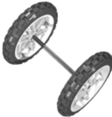
Figure 2.20 Two Connected Wheels Go Straight
